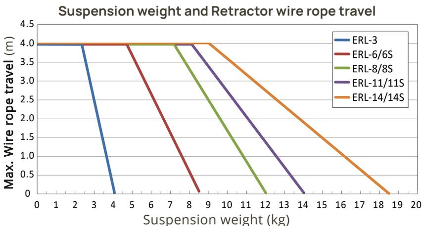
This graph shows the wire rope travel from the factory set position. This graph is a reference for straight up and down operation.
