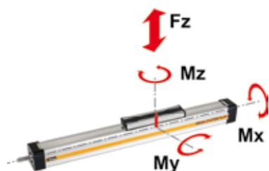
$$\begin{aligned}M &= F \cdot l \text{ [Nm]} \\M_x &= M_{x \text{ static}} + M_{x \text{ dynamic}} \\M_y &= M_{y \text{ static}} + M_{y \text{ dynamic}} \\M_z &= M_{z \text{ static}} + M_{z \text{ dynamic}}\end{aligned}$$
