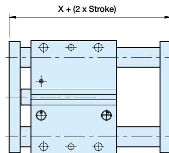
**Dimensions, P5T with two fixing plates and adjustable end stop with cushioning**
