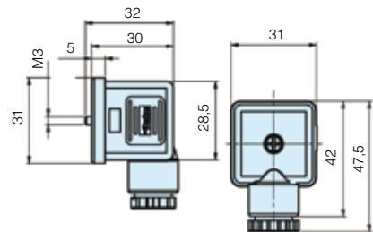
**EV310 Operator with 22 x 30 DIN form B coil****22 x 30 DIN form B connector**
