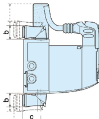
**Reminder :** peripheral modules may either be plugged in the valve output ports or mounted in line separate from the valve
