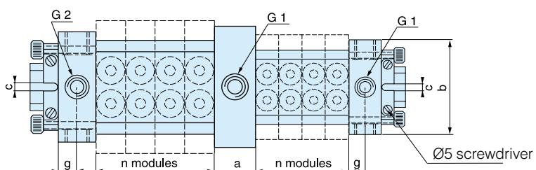
**Stacking power valves 1/4" with pneumatic or electrical control - With 1 W solenoid actuator and suitable pneumatic connector - Monostable PVL-C1216••, PVL-C1236••**
