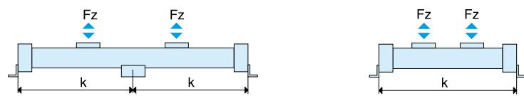
k = Maximum permissible distance between mountings/mid-section support for a given load F.
