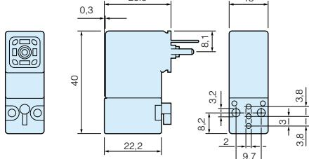
**Connector with standard screw**
