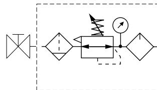
**Slide Valve + Filter/Regulator + Lubricator Combinations (50mg/m<sup>3</sup>)**
