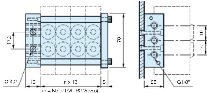
**Dual air supply – PVL-B1828**
