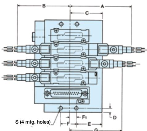
**A12P - Manifold - Side ports**
