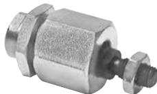
Flexo coupling for articulated mounting of piston rod. Flexo fitting is intended to take up axial angle errors within a range of  $\pm 4^\circ$ .
