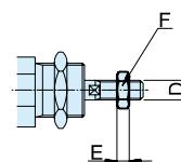
This range of stainless steel cylinders has been specially designed for use in difficult environments. Hygienic design, external seals of flourinated rubber and prelubrication with our food-industry-approved grease according to USDA-H1 make the cylinders particularly suitable for food industry use. All cylinders have magnetic pistons for proximity position sensing. Fixing dimensions to ISO 6431 simplify installation and make the cylinders physically interchangeable throughout the world.
