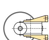
**Note:** Oil-bath gearboxes mean that the installation position must be decided in advance. The installation position determines the volume of oil in the gearbox and location of oil filling and drain plugs.
