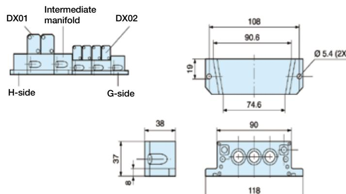
**ISO 5599-1 Subbase & Manifolds****VDMA Side Ported Subbases**
