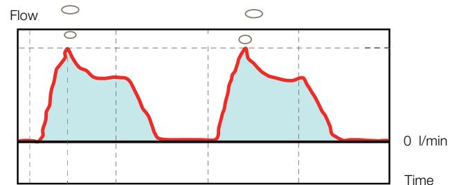
Compared to continuous air blow, the pulsed air blow hits the work repeatedly, improving the efficiency of the air blow.
