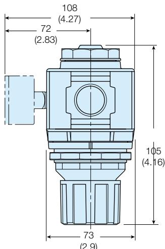
**NOTE:** Ø 60 mm hole required for panel nut mounting.
