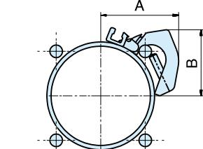
**Sensor mounting - P1D-T 160 - 320mm
