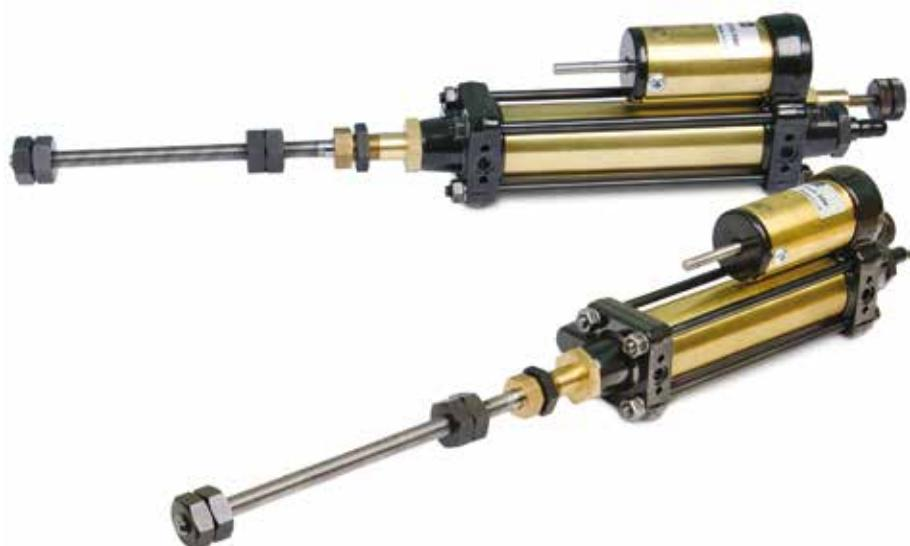
Hydrochecks are precision built self contained hydraulic control units designed to smooth out pneumatic cylinder movements over any distance within their own stroke length, up to 450 mm.
