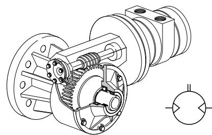
**F: Reversible motor with worm gear, flange mounting left-hand**
