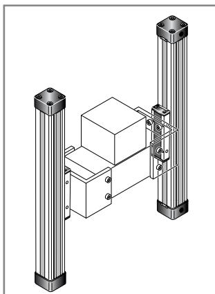
The mechanical design of the OSP-L allows synchronised movement of two cylinders.
