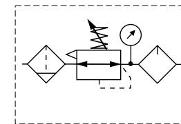
**Filter/Regulator + Lubricator Combinations (50mg/m<sup>3</sup>)**
