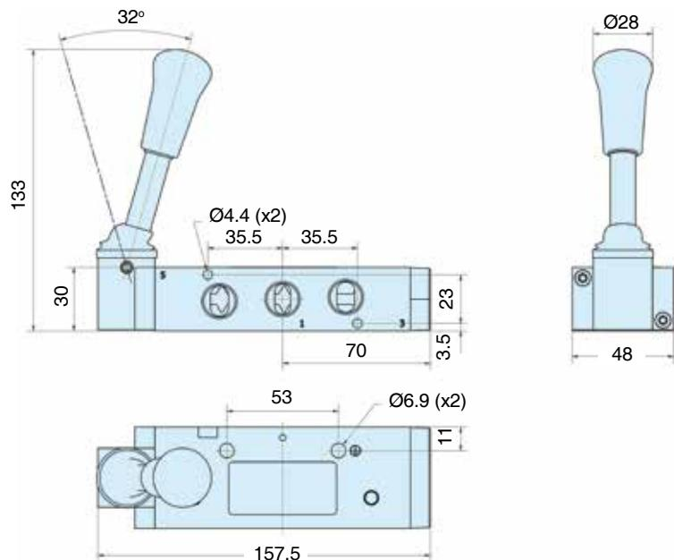
**P2LCX - 5/3 Lever operated directional control valves**
