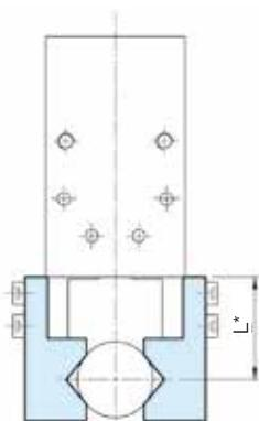
\* L = gripping joint length 30mm, pressure 5kgf/cm<sup>2</sup>
