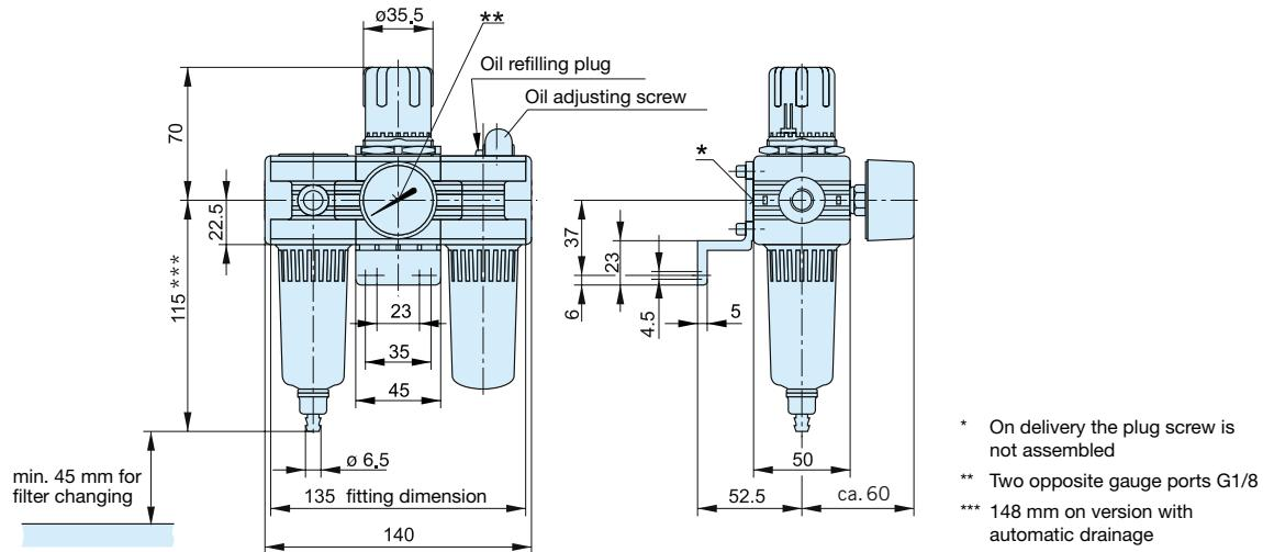
**Filter/Regulator + Lubricator combination**
