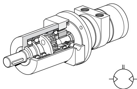
**B: Reversible motor with planetary gear, flange mounting, free installation position**
