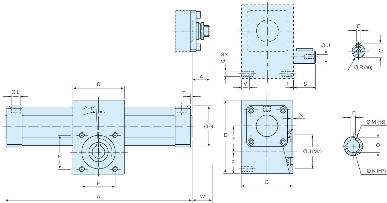
The location of the shaft key is indicated when the pistons are on the left.
