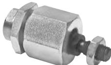
Flexo coupling for articulated mounting of piston rod. Flexo fitting is intended to take up axial angle errors within a range of  $\pm 4^\circ$ .
