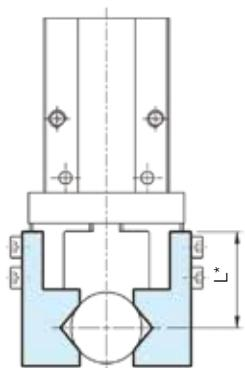
\* L = Gripping point L = 20mm at center of stroke
