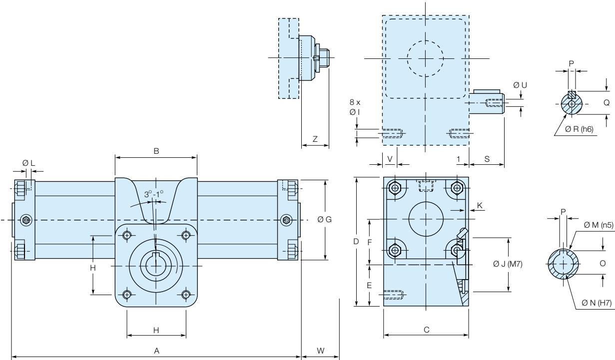
The location of the shaft key is indicated when the pistons are on the left.
