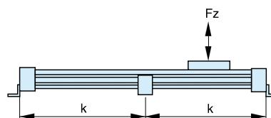
k = Maximum permissible distance between mountings/mid-section support for a given load F.
