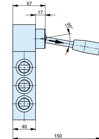
**5/3 Way Lever Operated Valves****G1/8 Hand lever actuated**
