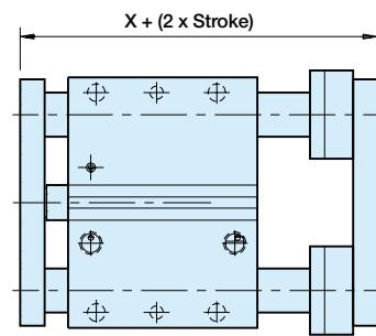
**Dimensions, P5T with adjustable end stop with cushioning**
