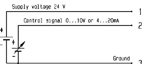
The female connector to mount is the 4 pole M12 connector (IEC 61076-2-101 model LF) where the pin number 4 is not connected.
