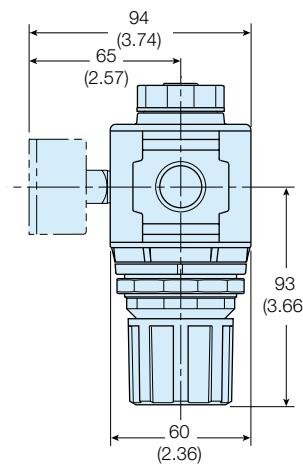
**NOTE:** Ø 30 mm hole required for panel nut mounting.
