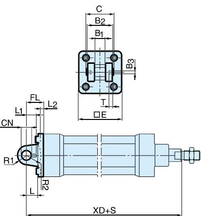
**Cylinder mountings****Pivot bracket with swivel bearing CS7**
