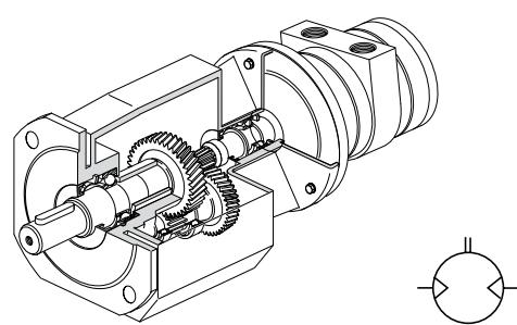
**D: Reversible motor with helical gear, flange mounting**
