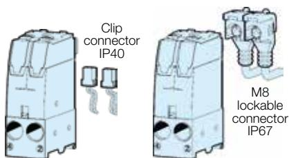
In its IP40 version, each solenoid shows Clip connection integrating LED and voltage surge protection. The clip connector with flying leads may be ordered separately with independent or interconnected common. In its IP67 version, each solenoid shows a M8 connection. Lockable connectors, IP67 protected, with LED voltage surge protection and flying lead cable may be ordered for the required length.
