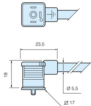
**Connector with large headed screw**
