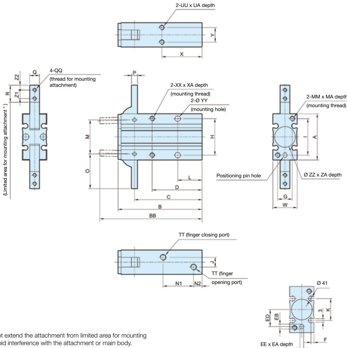
\* Do not extend the attachment from limited area for mounting to avoid interference with the attachment or main body.
