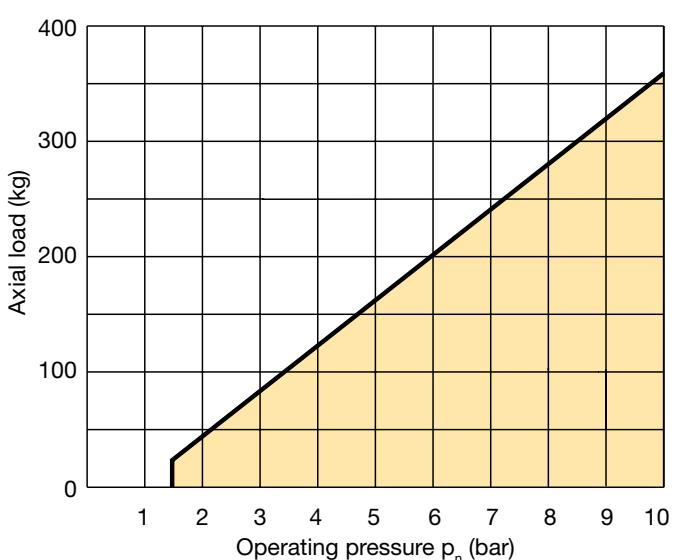
**STHSR Series - Stop cylinder Ø 50mm - Horizontal version****Order Key**
