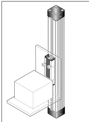
The high load capacity of the piston can cope with high bending moments without additional guides.
