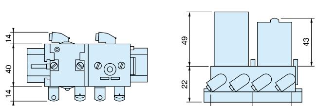
**Relays mounted on 3-port modular subbases**
