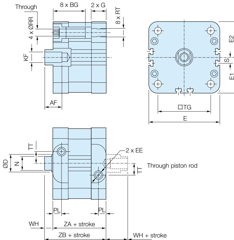
**P1PG...DS Double acting with guided piston rod**
