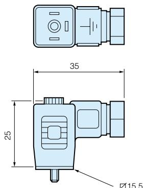
**CNOMO 22 x 30 solenoid operators and connectors****P2F Operator
