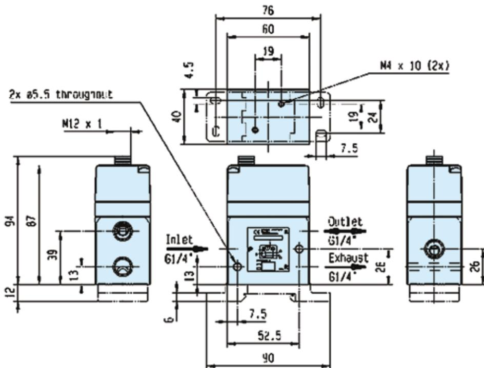
The male connector adopted on the EPP4 is a standard 4 pole M12, without the pin number 4:
