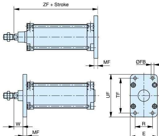
Dimensions for cylinders without piston rod protusion or with rod lock unit
