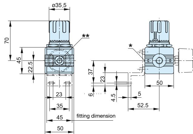
\* On delivery the plug screw is not assembled
