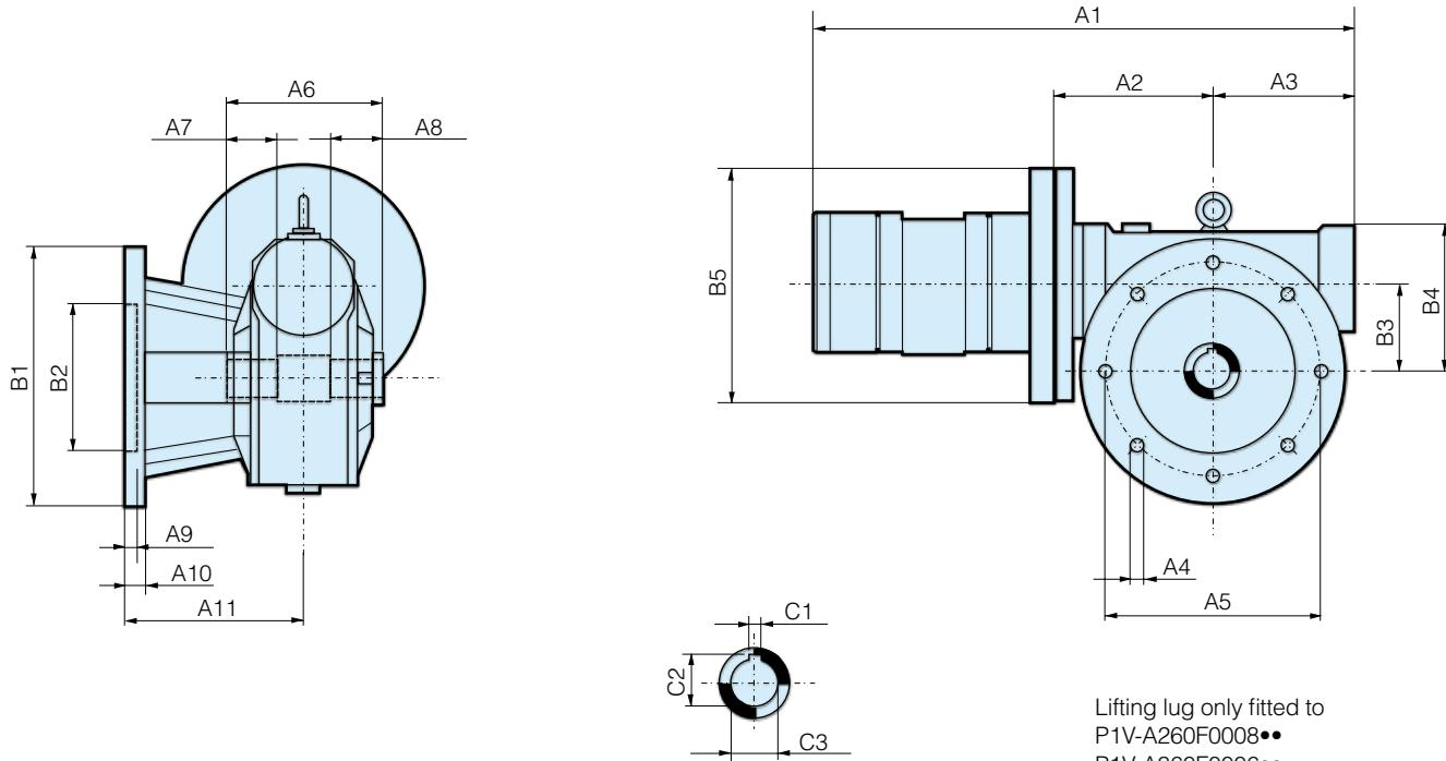
As standard, the motor has a hollow shaft with key slot. Please refer to page 44 for a dimension sketch of the single ended and double ended shafts and for additional flange on the opposite side.
