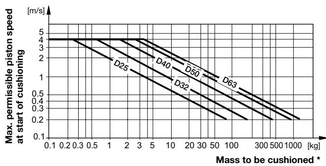
\* For cylinders with linear guides or brakes, please be sure to take the mass of the carriage or the brake housing into account.
