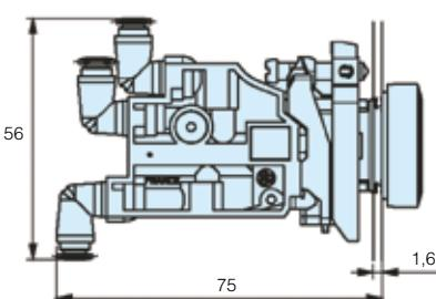
Compact 3/2 normally closed metal bodied valves with push-in air connections. Designed for the process duty cycle with high durability. Ideal for the process or packaging industry.
