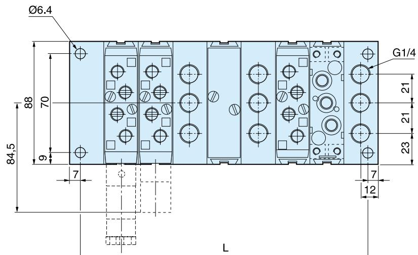
Connection block L and intermediate blocks L and T can be turned so that connection can be made from above or below.
