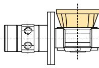
**Note:** Oil-bath gearboxes mean that the installation position must be decided in advance. The installation position determines the volume of oil in the gearbox and location of oil filling and drain plugs.
