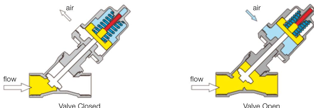
**PA Series - Compact Design Normally Closed Valves****Flow Direction OVER Seat**
