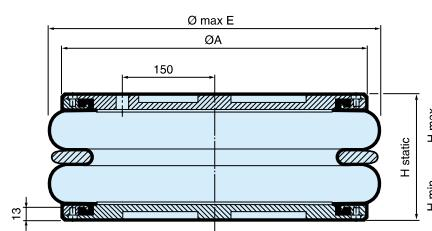
Air bellows are the ideal choice for applications requiring short stroke, high thrust single acting actuators.
