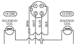
**H Series ISO 5599-1 - Sizes 1, 2 & 3****CNOMO operator with 30 x 30 DIN Form A / 24 Vdc / 2,7 W solenoid**
