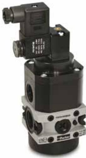
P3X Series Combined Soft Start/Dump Valves, provide for the safe introduction of pressure to machines or systems. Soft Start/Dump Valves when set, allow the pressure to gradually build to the set point before fully opening to deliver full flow at line pressure.
