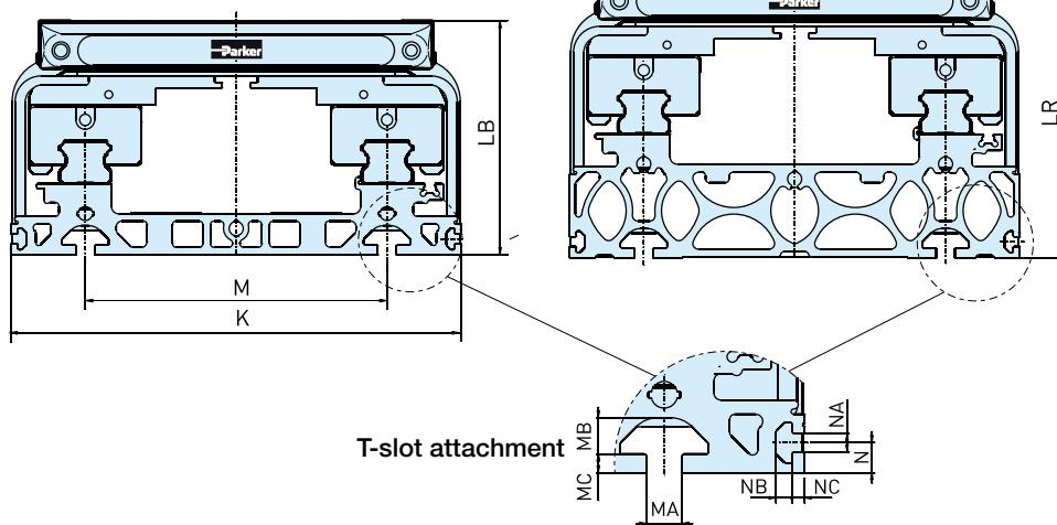
The HMR linear drive system can be equipped with a "basic" or "reinforced" profile as standard. The "basic" profile is suitable for fitting directly to a machine base that has a corresponding support surface. The "reinforced" profile, on the other hand, is the preferred choice for self-supporting systems or for use in conjunction with a base surface offering limited support.
