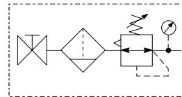
**Slide Valve + Filter/Regulator Combinations (50mg/m<sup>3</sup>)**
