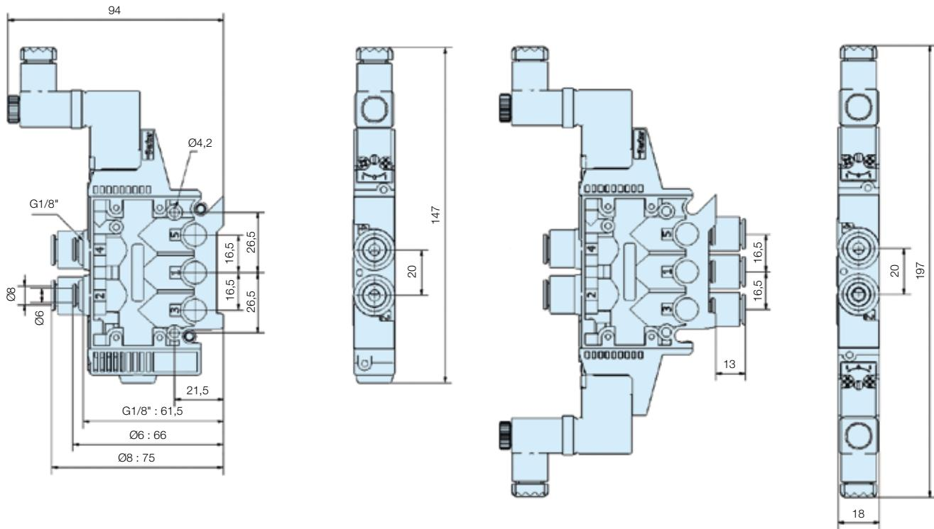
**PVL-B21 (Stand-alone) & PVL-B22 (Stackable) – with 15 mm pilot solenoid valve – Pins DOWN**
