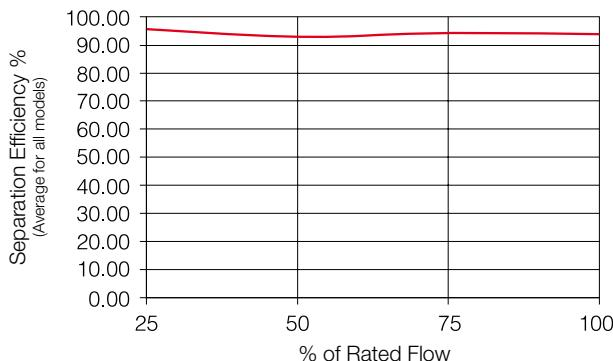
Tested with an inlet challenge concentration of 33ml/m<sup>3</sup>hr and in accordance with ISO 8573.9.
