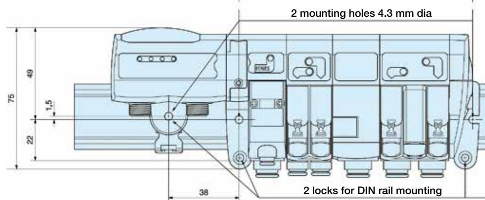
DIN rail 35x7 mm or 35x15 mm
