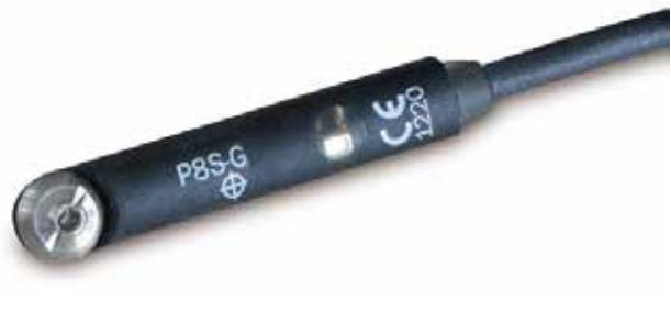
The P1D sensors can easily be installed from the side in the sensor groove, at any position along the piston stroke. The sensors are completely recessed and thus mechanically protected. Choose between electronic or reed sensors and several cable lengths and 8 mm and M12 connectors. The same standard sensors are used for all P1D versions.
