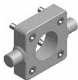
Intended for articulated mounting of cylinder. This trunnion can be flange mounted on the front or rear end cover of all P1D cylinders. At your choice, you can order a complete cylinder with factory-fitted flange mounted trunnion. Individual trunnions have order code as shown below.
