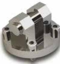
Intended for articulated mounting of cylinder versions D, F, or L. The bracket is mounted on the rear end cover and is supplied complete with shaft, mounting screw and O-ring for a clean joint between end cover and bracket.
