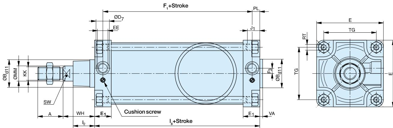
**Note:** for bore size 320mm, front air port in on the bottom of the axis of the cylinder and the cushioning screw on the top
