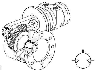
**G: Reversible motor with worm gear, flange mounting right-hand**
