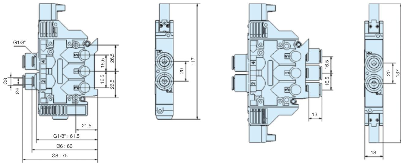
**PVL-B21 (Stand-alone) & PVL-B22 (Stackable) – with 10 mm pilot solenoid valve – Pins UP**
