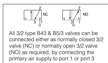
All 3/2 type B43 & B5/3 valves can be connected either as normally closed 3/2 valve (NC) or normally open 3/2 valve (NO) as required, by connecting the primary air supply to port 1 or port 3
