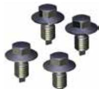
Set of 4 threaded plugs to be fitted in unused end cover screws. A rubber gasket is supplied with every plug. The seal off function is equal to IP67. The plugs can be used for all P1D cylinders to avoid collecting dirt and fluids in the end cover screw recesses.
