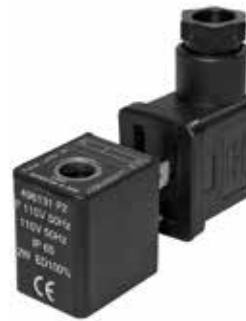
496637 coil series with connection 2P + G when mounted together with the supplied Pg9 plug (delivered with the coil) are suitable for use in dangerous areas (dust Zone 22) according to the European directive ATEX 94/9/C. Protection mode: Ex tD A22 IP65 - T95°C
