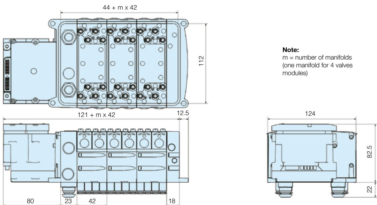
High speed poppet type solenoid valves with individual electrical connections. Light weight plastic bodies with DIN rail manifold. Ideal for cabinet installations.
