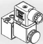
The standard valve is fitted with a 30mm solenoid having DIN 43650 Industrial form A connector for sizes 1, 2 and 3 15mm solenoid for sizes 01 and 02.
